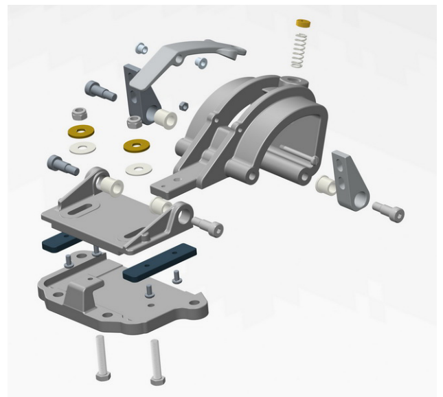
BFHHQTH-HINGE Exploded View
